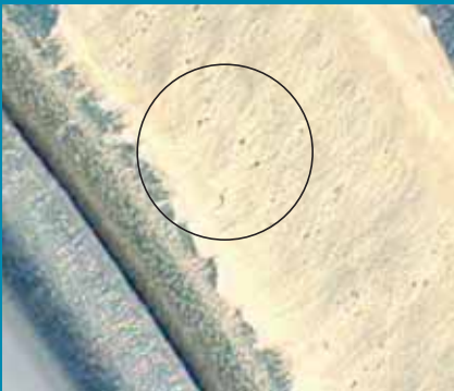
Sealed area of heat seal lacquered ring: showing voids
